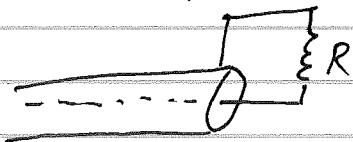
A transmission line (like a coaxial cable) can be "impedance matched" to a resistor  $R$  so that all power incident on the resistor is absorbed; when matched, the transmission line has the same impedance as the resistor. Thus the resistor is in effect a "black body" — in thermal equilibrium it radiates at the same rate it absorbs, so the rate at which the resistor dissipates power must agree with the rate at which the transmission line delivers power to the resistor.
