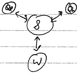
work  $Q_h - Q_c$  is done by reversible engine.  $Q_h$  withdrawn from hot reservoir
