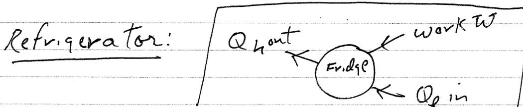
A refrigerator is a heat engine run backwards: instead of using the flow of heat from hot to cold to do work, it uses work to pump heat from a cold place to a hot place. Its performance is measured by  $\gamma = Q_c/W$  - the heat removed per unit of work
