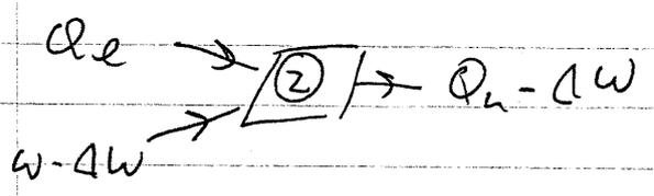
But as a refrigerator, (2) is no more efficient, because it removes  $Q_c$  from cold reservoir, doing less work
