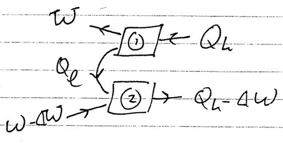
Now use the refrigerator to pump waste heat back to the hot reservoir.
