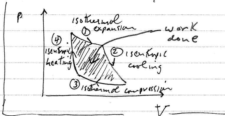
The area enclosed by the curves the difference between work the gas does during expansion, and work we do during compression.
